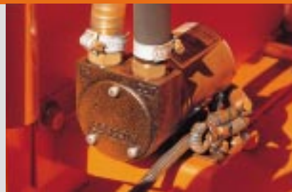
Electric fuel supply pump
