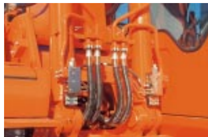
Boom and arm hose rupture protection valve
