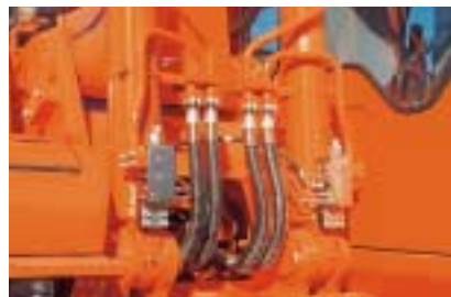
Boom and arm hose rupture protection valve
