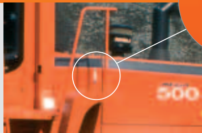
An oil level indicator at the centre of the machine is clearly visible.
