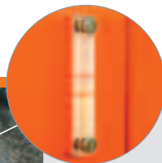
An oil level indicator at the centre of the machine is clearly visible.
