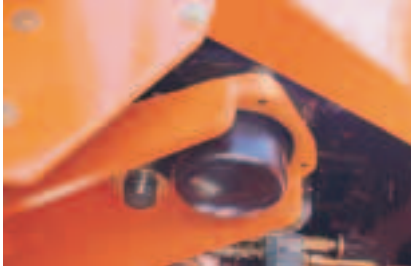
Viscous hydraulic suspension mounts reduce moving vibrations within the cab.
