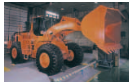
Rolling conditions simulations (braking, acceleration, drawbar pull, heat dissipation...).
