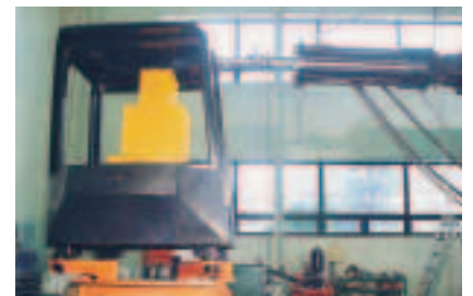
Cab tests according to Fops and Rops norms.
