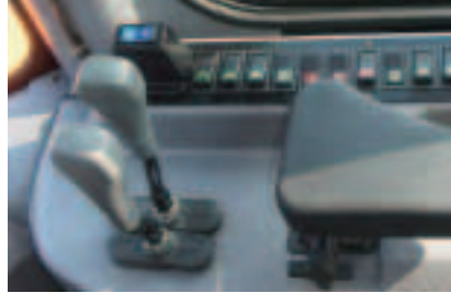
The selection of forward and reverse is integrated into the two hydraulic control levers. (option)
