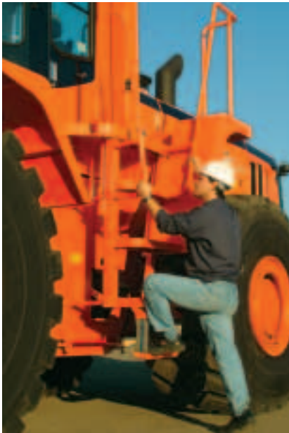
Accessibility is both simple and safe. For greater comfort, the steps are inclined, with hand and guard-rails ergonomically placed for safe climbing, inspection and disembarking.
