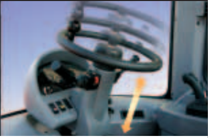
The steering column features both tilting and telescopic adjustment.
