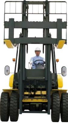
Superb forward visibility Elimination of the intermediate mast cross member improves visability when loading. Masts are painted unobtrusive grey and the forks hi-visability yellow.
