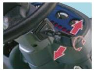
Electrically controlled forward-reverse direction lever provides finger tip control Reducing the force required to shift
