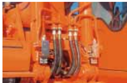
Boom and arm hose rupture protection valve
