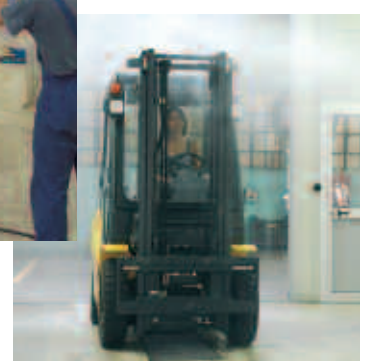
Waterproof design. The plastic parts are shaped to shed water while the electrical connections are all waterproof. The levers and controls are all amply protected with special trim seals
