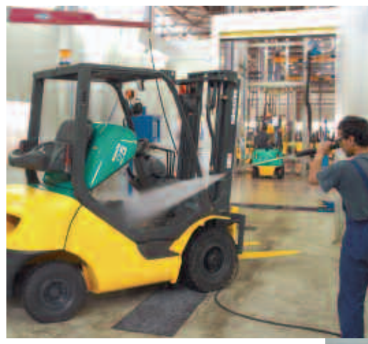
Waterproof design. The plastic parts are shaped to shed water while the electrical connections are all waterproof. The levers and controls are all amply protected with special trim seals
